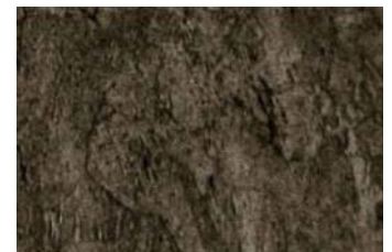
Luvata CuCrZr fine grain structure
