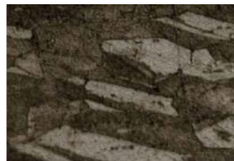
Conventional CuCrZr grain structure
